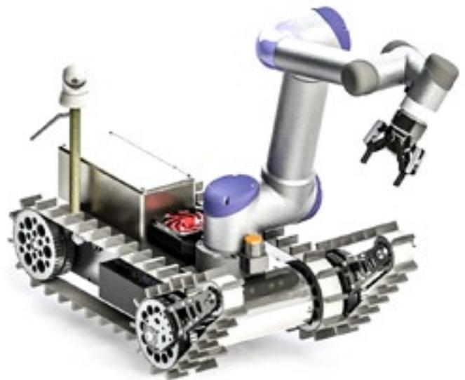
The arm gripper is interchangeable, among other tools it can mount gripper/plier cutter adapter, interchangeable gripper fingers, rotary multi-tool (drill, saw, impact driver, reciprocating saw, router, etc.). The controller allows cartesian TCP motion commands.
